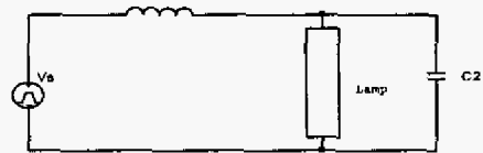
Fig. 1a Practical electronic ballast configuration
