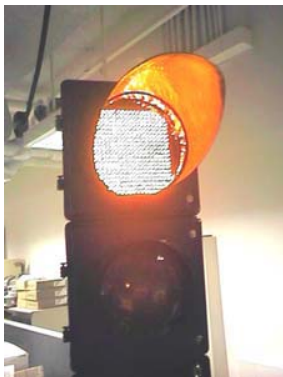
Fig. 3 Photograph of the LED traffic light.
