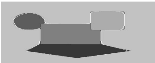
Figure 2b. The outline obtained using B-Spline snakes. Some of the hard corners are not fitted perfectly.
