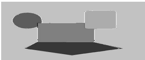
Figure 2c. The outline obtained using the two-stage B-Spline snakes approach. Many more of the hard corners have been fitted perfectly.
