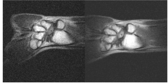
Fig. 7. Comparison sagittal image of the wrist [2.5-in copper coil (left) versus 2.5-in HTS coil (right)]. SNR gain 2.62.
