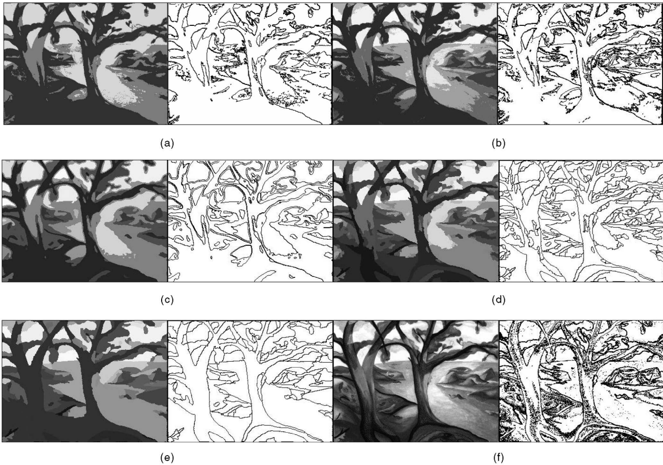
Fig. 9. Segmented images and region maps of "Trees" according to smallest L . (a) KMC. (b) CGC. (c) SRG. (d) QBS. (e) Proposed. (f) Original.
