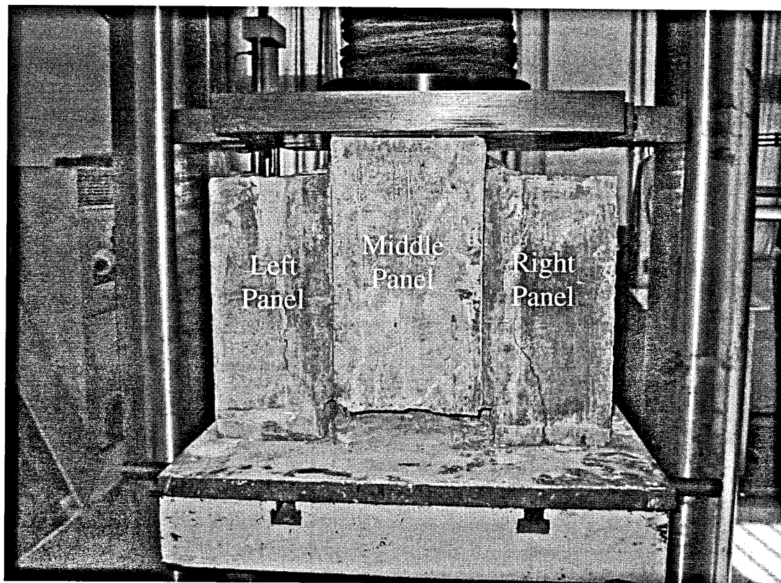
Fig. 12. Laboratory setup for testing the connection strength of three concrete panels.
