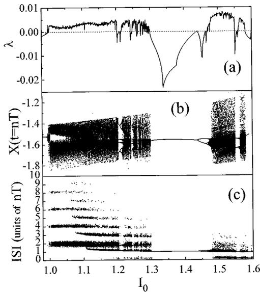
FIG. 3. The dynamical characteristics of a neuron as a function of  $I_0$  [a weak periodic signal  $I_1 \sin(2\pi f_s t)$  with  $I_1 = 0.1$  and  $f_s = 40$  Hz has been used]. (a) The maximum Lyapunov exponent  $\lambda$ ; (b) the projection of potential  $X(t)$  at time  $t = nT_s = n2\pi/f_s$ ; (c) the interspike interval ISI (with units of the period  $T_s$  of the signal).
