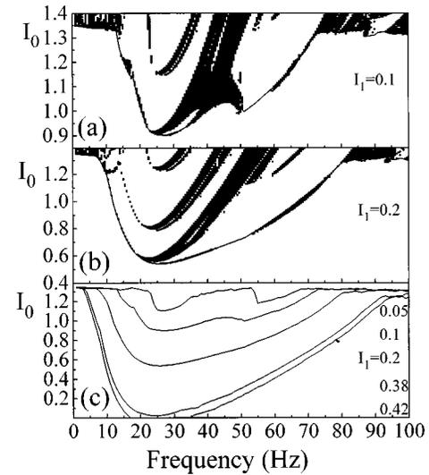
FIG. 4. The phase diagram of different dynamical behaviors in constant stimulus  $I_0$  against the signal frequency  $f_s$  for different amplitudes  $I_1$  of the signal. (a) and (b), the points represent the Lyapunov exponent  $\lambda > 0$ , a chaotic firing of spikes. The blank regions represent periodic firing with  $\lambda < 0$  (above the enveloped line) or nonfiring (below the enveloped line); (c) different enveloped lines for different values of the amplitude  $I_1$ .
