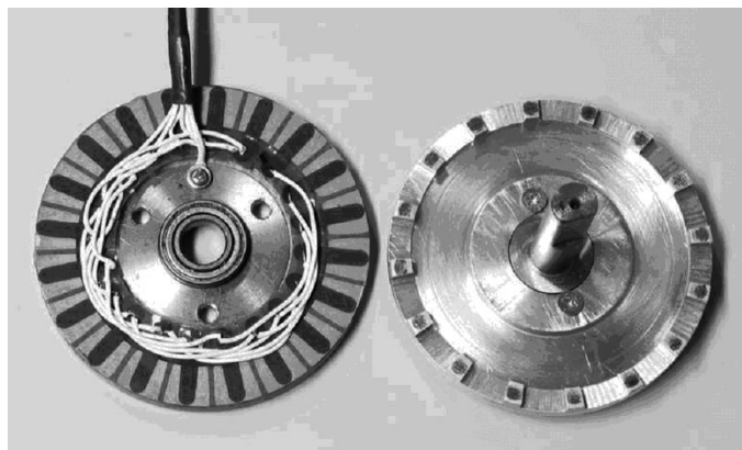
Fig. 5. Prototype of 80-step USM (left: stator; right: rotor).
