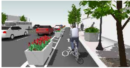
... With planters separating the bike lane
