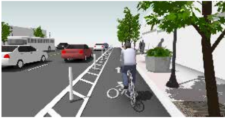
... With a 2-3 foot buffer and plastic flexposts
