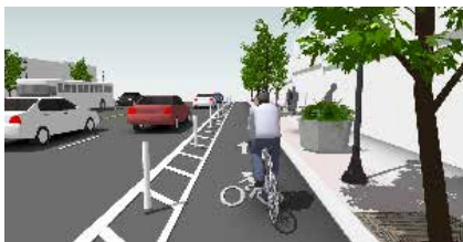
... With a 2-3 foot buffer and plastic flexposts
