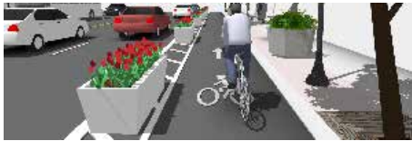
... With planters separating the bike lane
