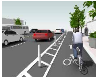
(D) On a similar street to (B), but with a physically separated bikeway
