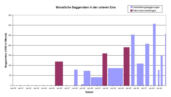
Figure 3.3: Monthly dredging rates in the Ems between Emden and Pappenburg between 1980 and 2000, in units of 1000 m<sup>3</sup>/month. The magenta refers to deepening of the channel, while the blue denotes maintenance dredging. Adapted from Habermann, 2003.
