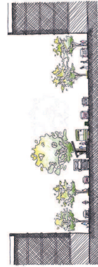
Option 3: 140'-6" right of way allows for one BRT lane, two side-access lanes and four through lanes
