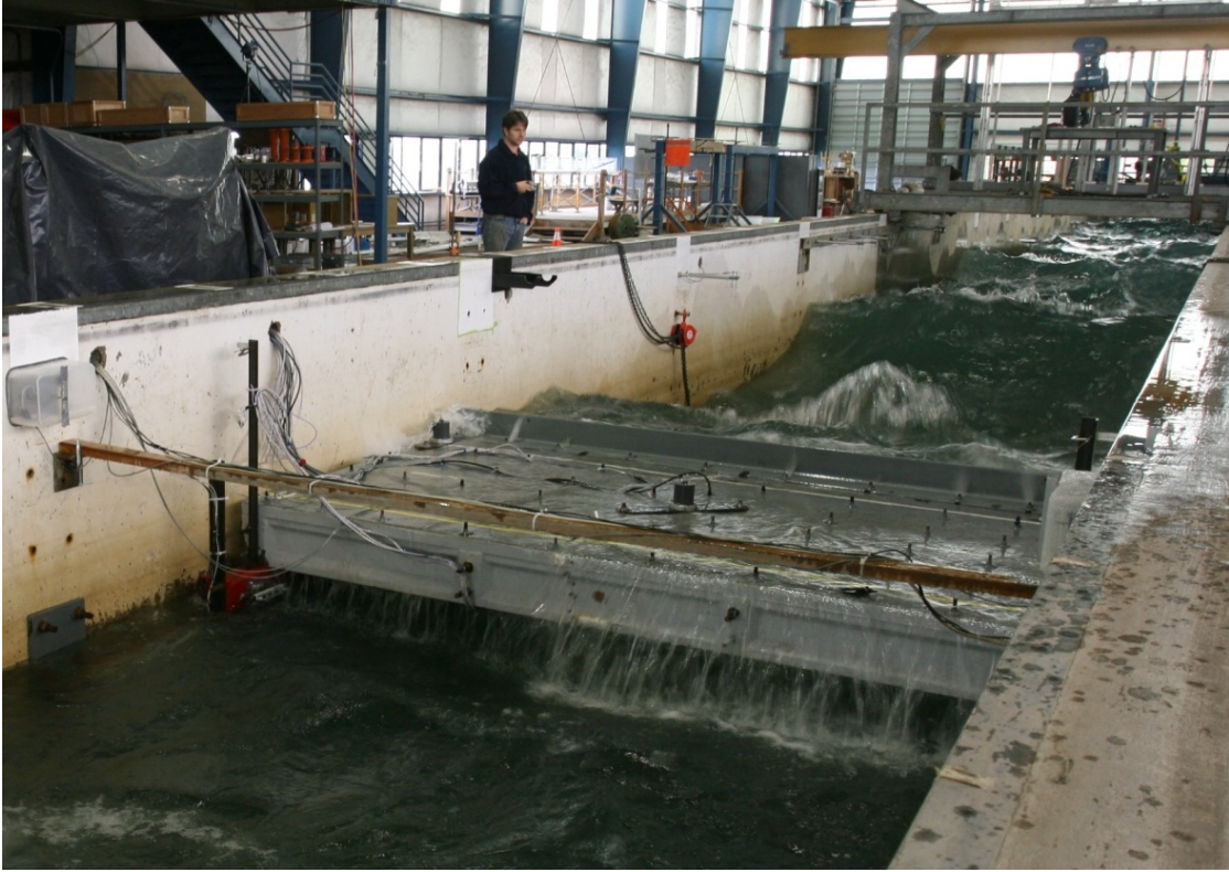
Figure 4.5. Photo of the bridge specimen during random wave trial at d^* = 0 .
