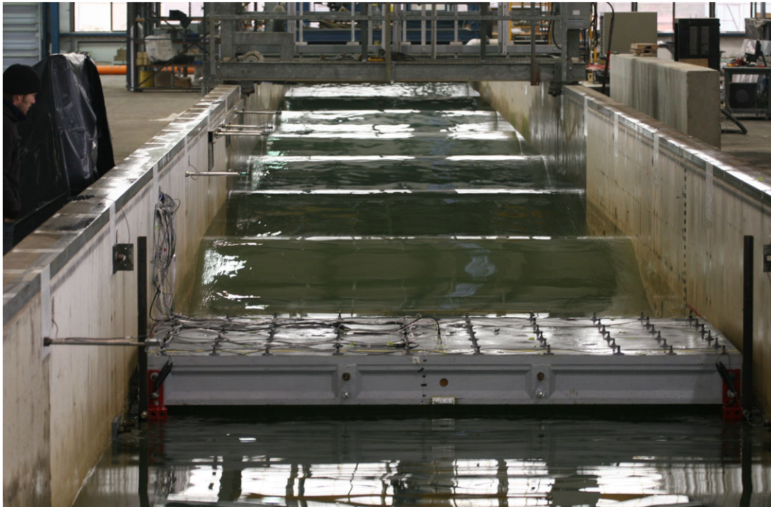
Figure 4.1. Photo of the bridge specimen during regular wave trial at d^* = 0 .
