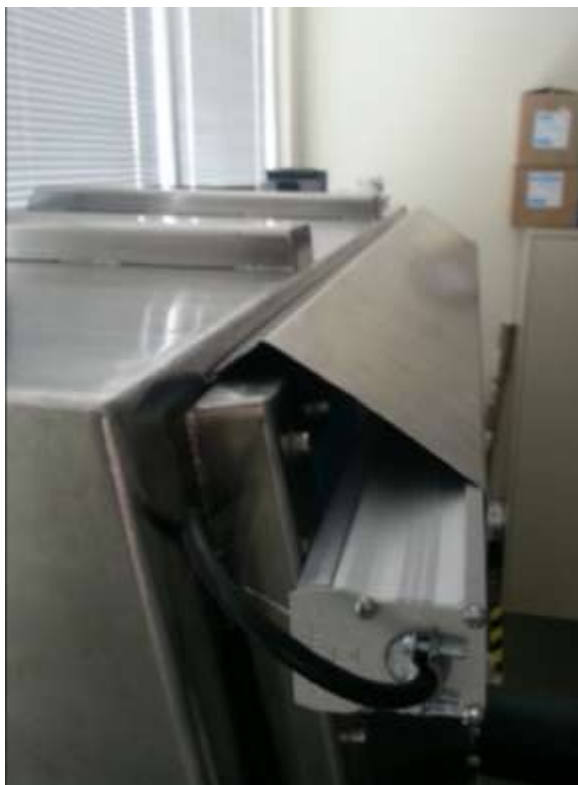
Figure 2.11: Light fixture for the glove box.
