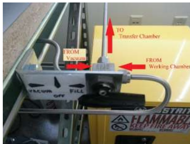
Figure 2.8: Three-way valve used to manually control the transfer chamber pressure. Currently allowing the flow from the vacuum pump to the transfer chamber.
