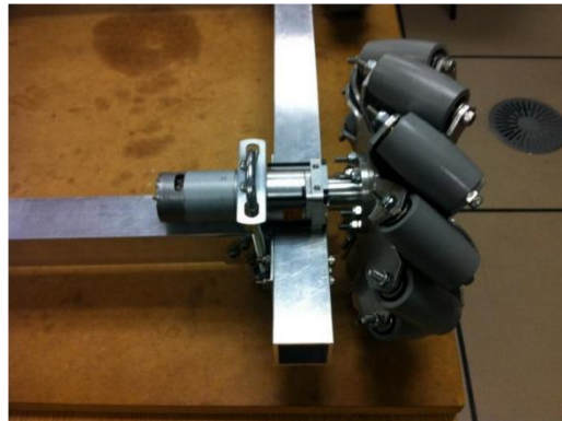
Figure 5.51: Mecanum wheel is connected to the gearbox and DC motor and mounted on the aluminum bar.
