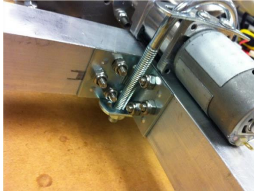
Figure 5.52: U shape bolt holds the gearbox to the main frame.
