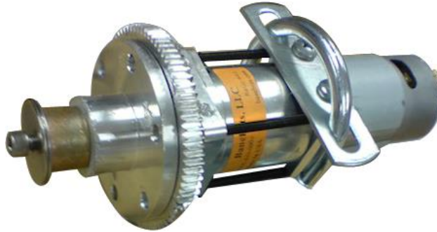
Figure 5.16: Motor spacer and its holding washer.
