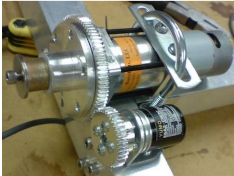
Figure 5.12: U shape bolt is used to attach the DC motor and its gear to the main frame.
