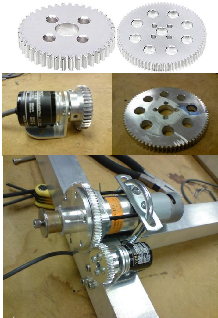
Figure 5.26: gears to attach the encoder to the gear shaft.
