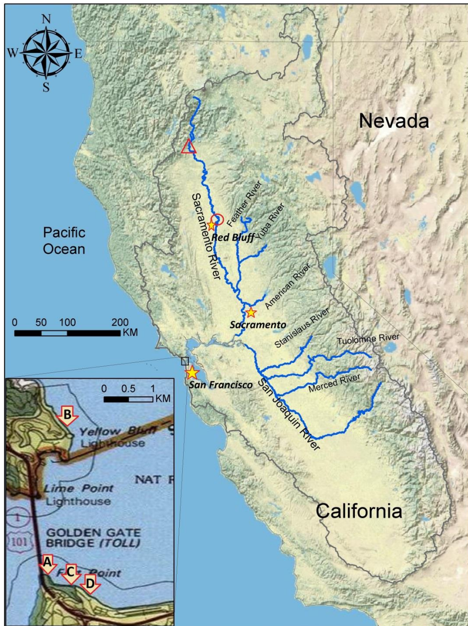
Figure 2-2: San Francisco Bay delta watershed boundaries and tributaries (USGS, HUC, http://www.nationalatlas.gov/ ); points A, B, C and D show tide gage locations (NOAA Station ID: 9414290) at Fort Point (1854 – 1877), Sausalito (1877 – 1897), Presidio (1897 – 1927) and Presidio (1927 – present), respectively. The red circle shows the stream gauge site for Sacramento River near Red Bluff (USGS 11377100); the red triangle indicates the Shasta Dam (©ESRI).
