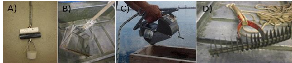
Figure 1: Sampling equipment for juvenile and adult Dreissena including A) Portland Sampler, B) surface scraper, C) grab sampler, and D) thatch plant rake on rope.
