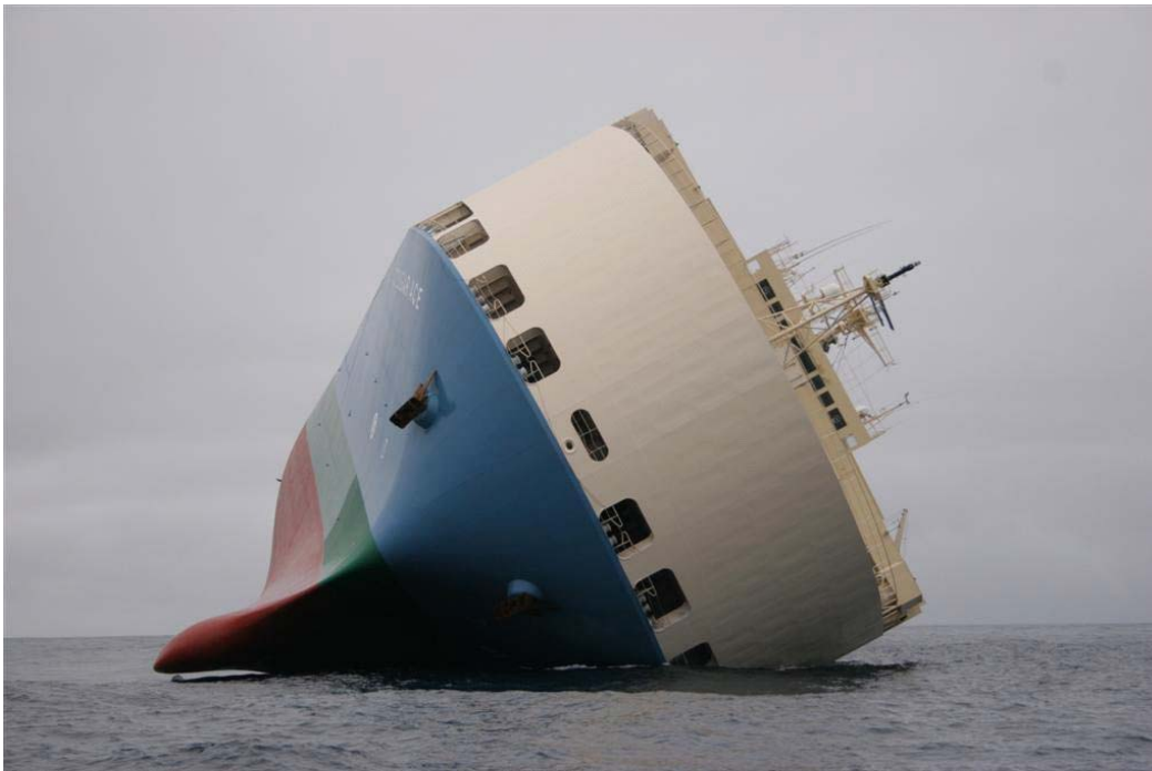
Figure 1: M/V Cougar Ace listing to port following ballast water adjustment. (Photograph by: The Associated Press)
