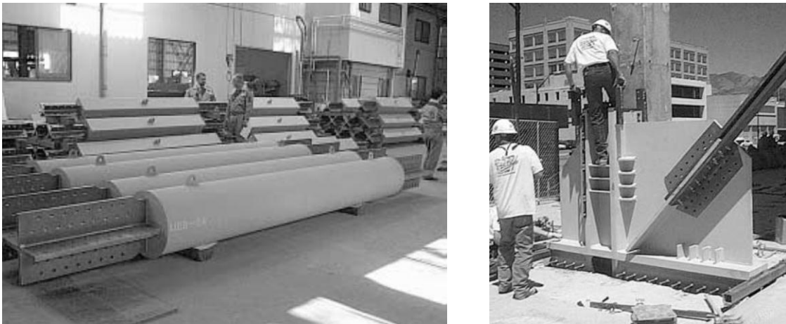
Figure 4 - BRBs at manufacturing facility in China and gusset plates on site (Brown et al., 2001)
