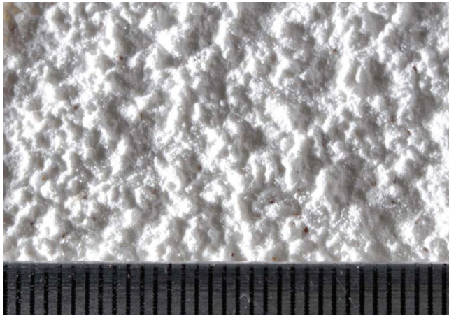
FIG. 4. (Color online) Photo of a lactose pellet impressed with a 40 grit rough surface. The width of the sample in the photo is 3.4 cm, (divisions in mm).
