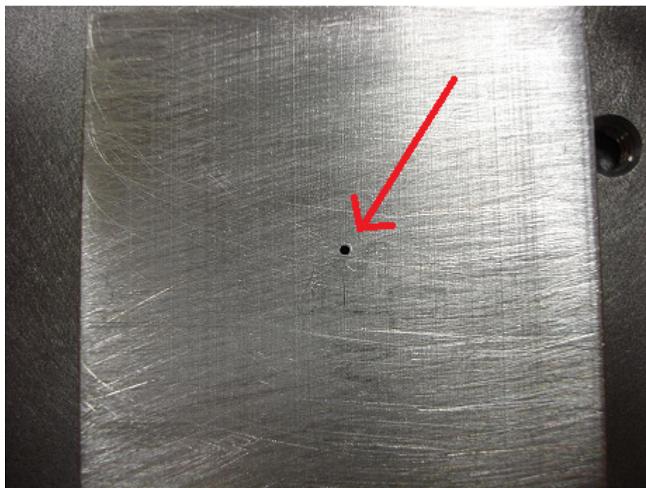
Figure III.8: PPW side of conical plates in figure III.7 with input/output hole marked
