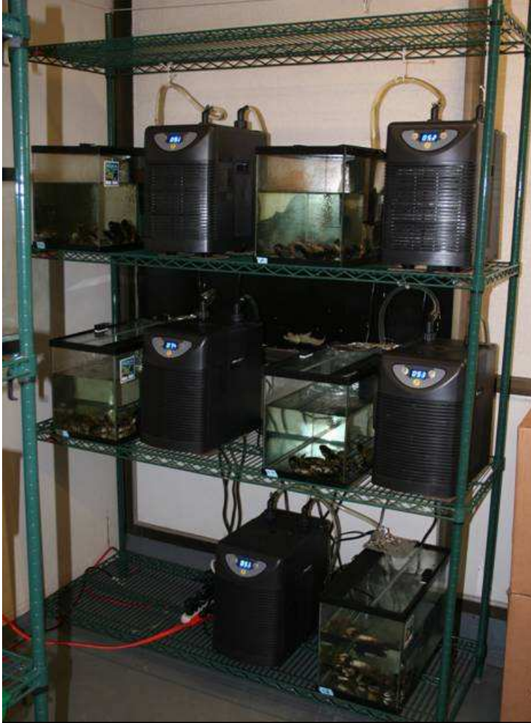
Figure 3.2: Experimental tanks. Tanks were connected to in-line chillers and the temperature maintained at 10°-11C.
