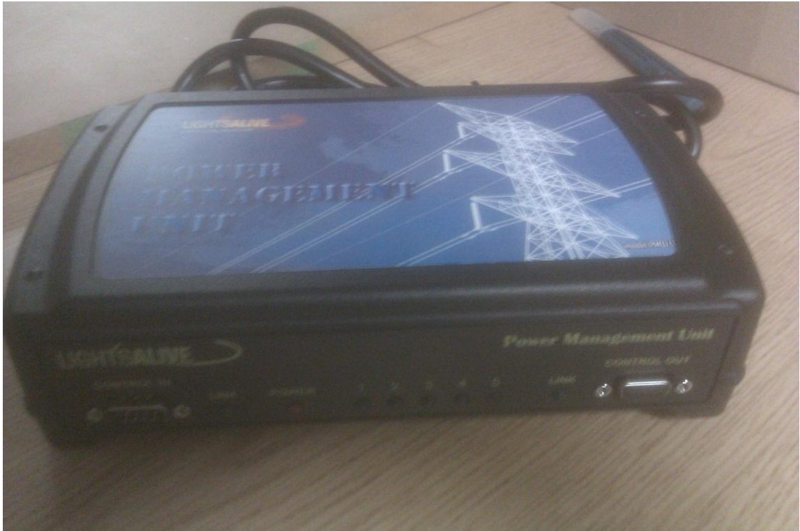
Figure 5:2 Power Management Unit for Chameleon Musical Light Controller
