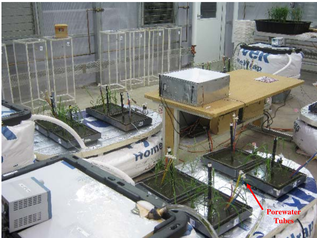
Fig. 4.2: Pictures of pore water tubes embedded into flooded soils inside tubs containing temperature probes. The tubes were fitted with valves to which the syringes were hooked during sampling.
