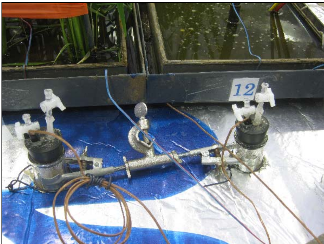
Fig. 5.2: Picture of production jars mounted onto the water bath system. The jars are fitted with valves and thermocouples connected to microloggers (not shown in picture). Temperature was continuously monitored and recorded every 5 minutes during the growing season. The glass jars were purged with N_2 several times before each sample was collected.
