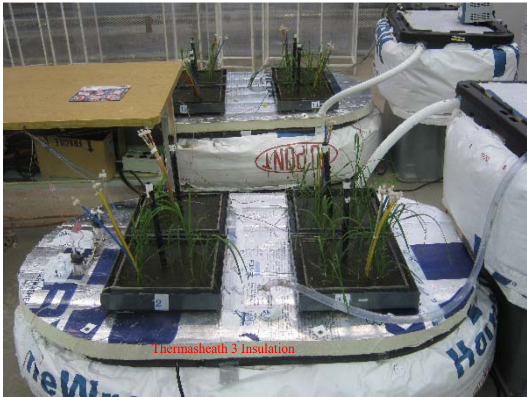
Fig. 2.2: Water bath and heating tanks were thermally insulated using fiberglass material. The top of water bath containers covered with Thermasheath 3 Insulation material to reduce heat loss.
