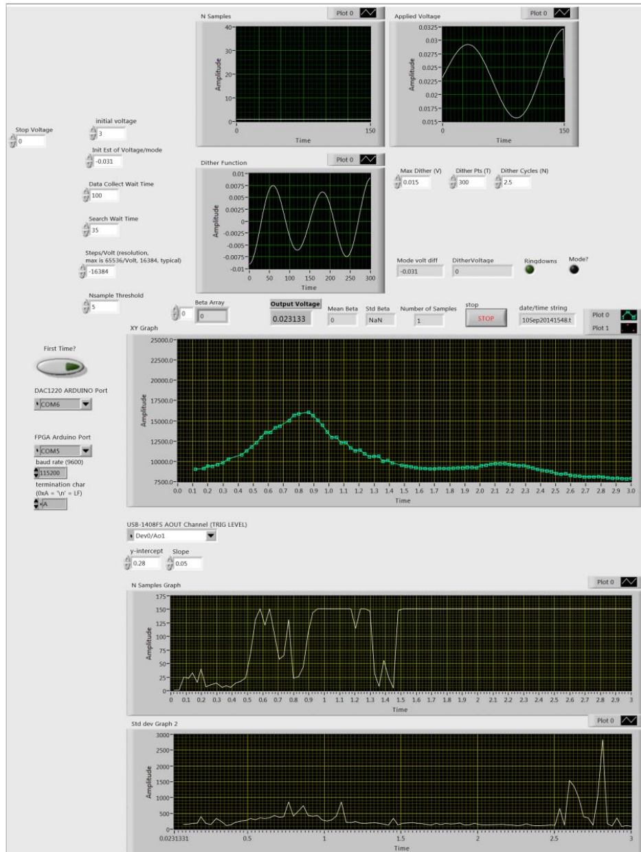
Figure F-1. User interface for the LabView code which controls the CRDS system and collects the data.
