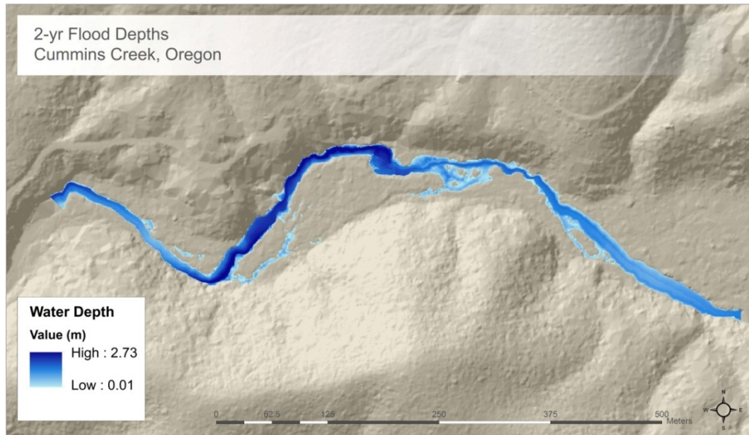
Figure 4.8: 2-year Water Depth Map at Cummins Creek, OR. Resulting values are rounded to the hundredth to set a minimum depth of 1mm. Values less than 1cm were set as null values.
