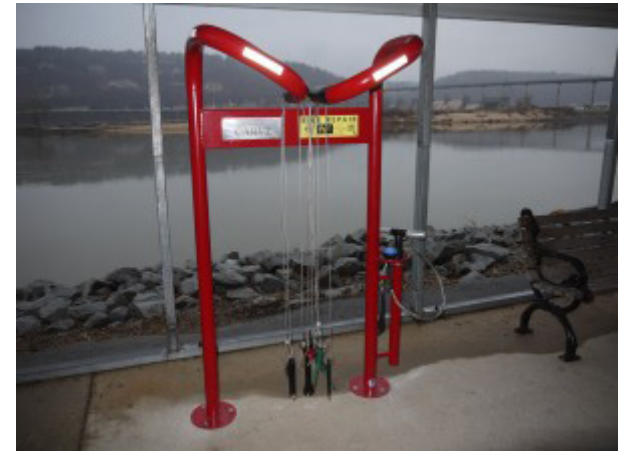
Public bike repair stations, like this one in Little Rock, Arkansas, provide essential tools for visiting cyclists to do minor repairs. (photo credit: Mason Ellis, Life in the Rock)
