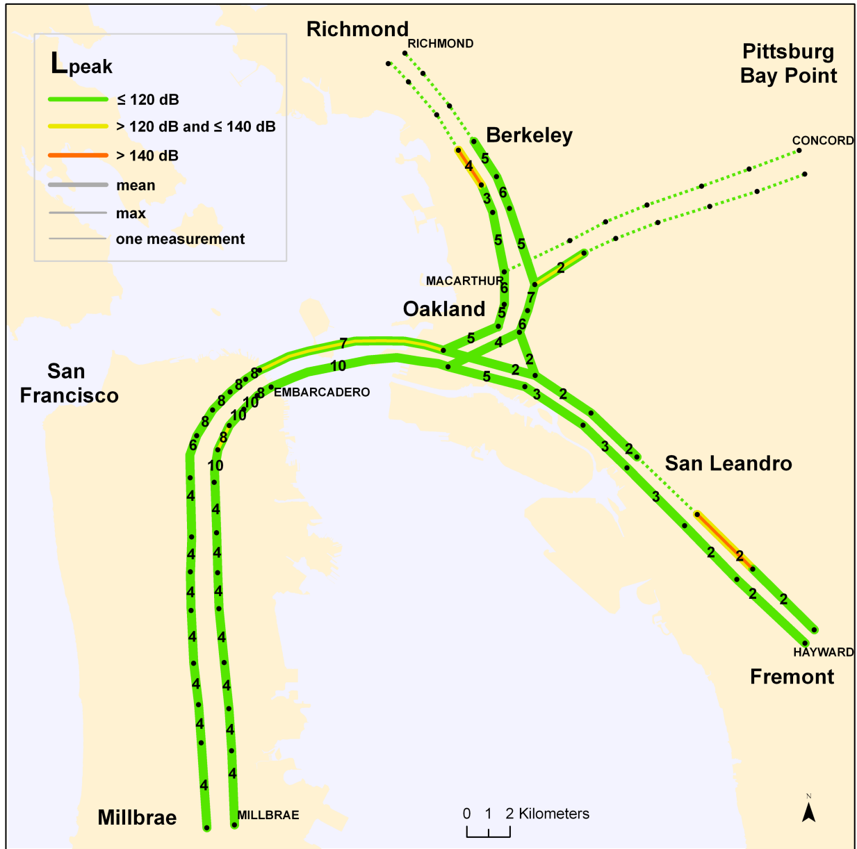
Figure 2 Map of mean and maximum L_{peak} (dB). The number of observations is overlaid on each line segment except those with a single measurement. The shape and position of line segments have been distorted to facilitate visual discrimination, and should be interpreted as schematic.
