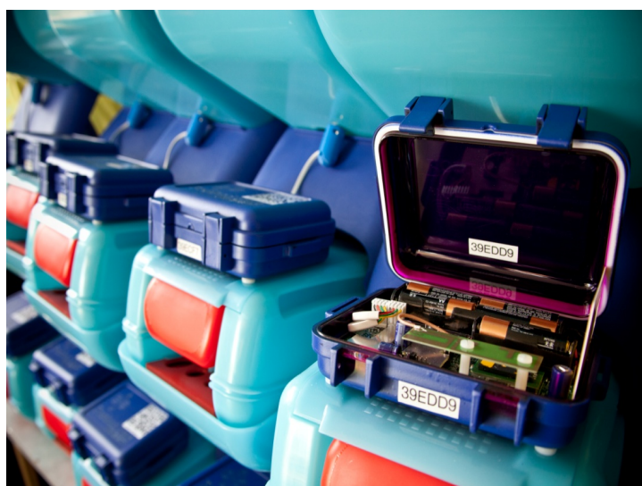
Figure 2. Sensors on household water filter. The dark blue waterproof box contains the electronics board. Pressure transducers are routed from the box (white cable) to the input bucket of the water filter.
