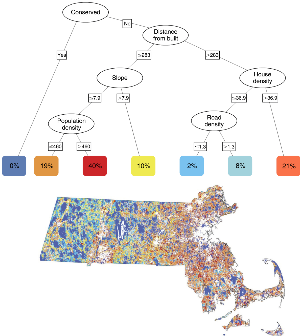
FIG. 4. Regression tree used to create probability (color-coded percentages) of future forest conversion zones used within the LANDIS-II simulations. The regression tree model used the pattern of forest conversion observed in the period spanning 1985–1999 in relation to the predictor variables described in Table 3. Terminal nodes of regression trees were scaled by their area on the landscape and were used to spatially allocate forest conversion within simulations. Units for the predictor variables are given in Table 3.
