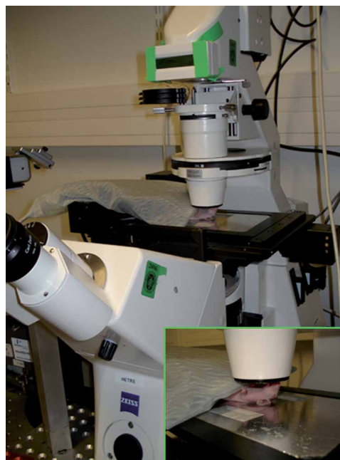
Figure 2 | Experimental setup for imaging sporozoites in the dermis of the murine ear. Once the mouse has been bitten, it is placed on the microscope platform so that the site of bite (on the ear) is in the middle of the coverslip over the hole. The ear is then taped into place to avoid any displacement during recording, and the mouse is covered with the homeothermic blanket.
