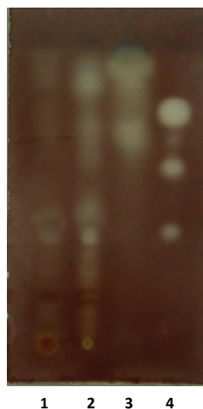
Figure 1. TLC qualitative acetylcholinesterase assay. 1. EtOH crude extract (200 \mu\text{g} ); 2. Alkaloid fraction (100 \mu\text{g} ); 3. Hexane fraction (100 \mu\text{g} ), and 4. Physostigmine (0.05 \mu\text{g} ). TLC elution system: \text{CHCl}_3:\text{MeOH}:\text{NH}_4\text{OH} , 90:7.5:2.5 v/v.
