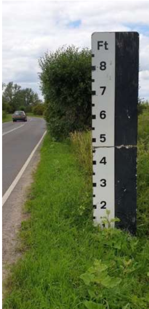
Figure 14: Flood water gauge board on a road crossing the Ouse Washes near Welney, Cambridgeshire. (Photo – S. Page).
