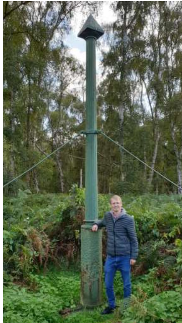
Figure 2: The Holme Post at Holme Fen, Cambridgeshire. In 1851, a metal post was driven into the peat so that its top was level with the ground. The top of the post is now some 4 m above the land surface, and at 3 m below sea level, Holme Fen is the lowest point in Britain. (Photo – S. Page).
