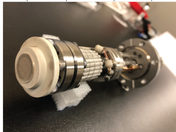
Fig. 2: Operation mechanism of ROAR's atomic oxygen source (top). Picture of the AO source before mounting it into the main chamber (bottom).
