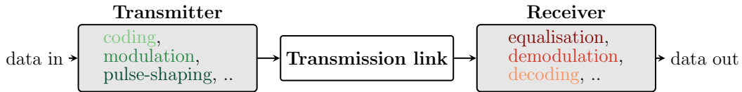
Figure 1.2: Basic schematic of a conventional communication system design, showing some of the main signal processing modules at the transmitter and the receiver.
