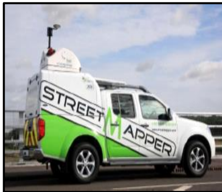
Figure 5-9 Kinematic Laser Scanner (Mazzanti, 2016)
