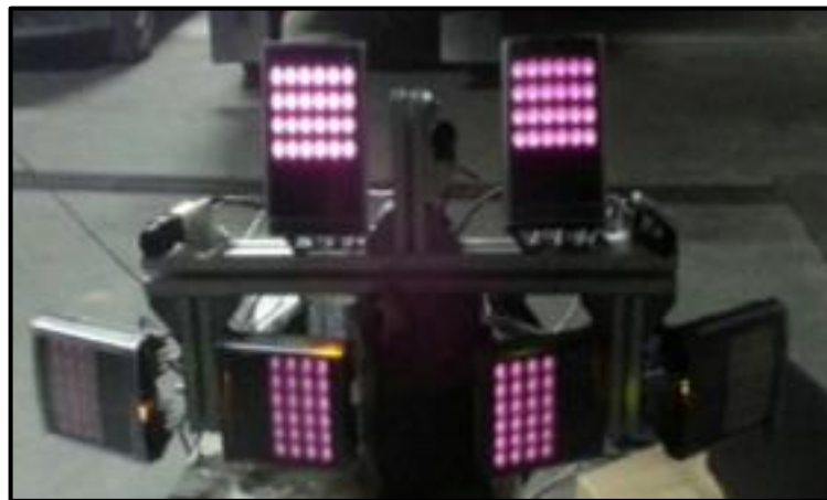
Figure 3-23 Set of illuminators and Infrared Cameras (Euroconsult, 2016)
