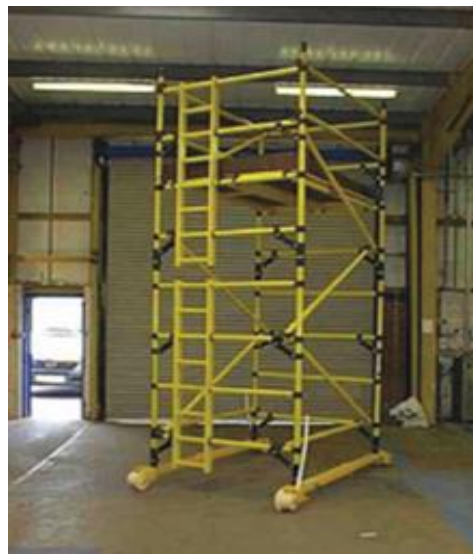
Figure 3-60 Rotamag tower set-up used for visual inspection (Permaquip, 2016)
