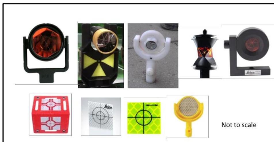
Figure 5-4 Examples of prism (top) and retroreflective targets (bottom) used with total stations (Soni, 2016)
