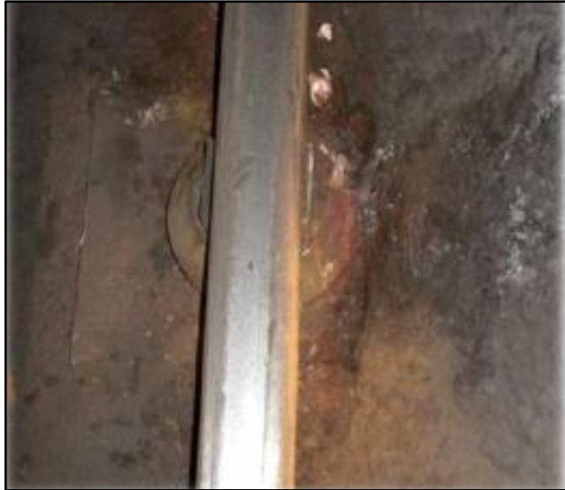
Figure 2-4 Water ingress; short circuit – earth fault or Burning (A2)
