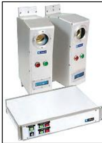
Figure 3-17 Laser-camera units/laser line projector and digital scanning camera (Euroconsult, 2016)
