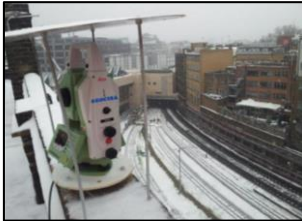
Figure 5-3 Total Station on fixed location for deformation monitoring (image from Geodata )
