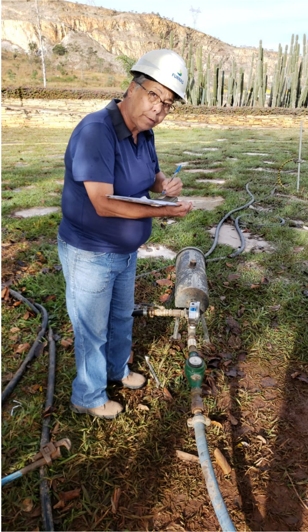
Figure 1 - Mother at Furnas Hydropower Dam. Performing “water loss test with drilling rig”. Credit: Personal archive. July 2019.
