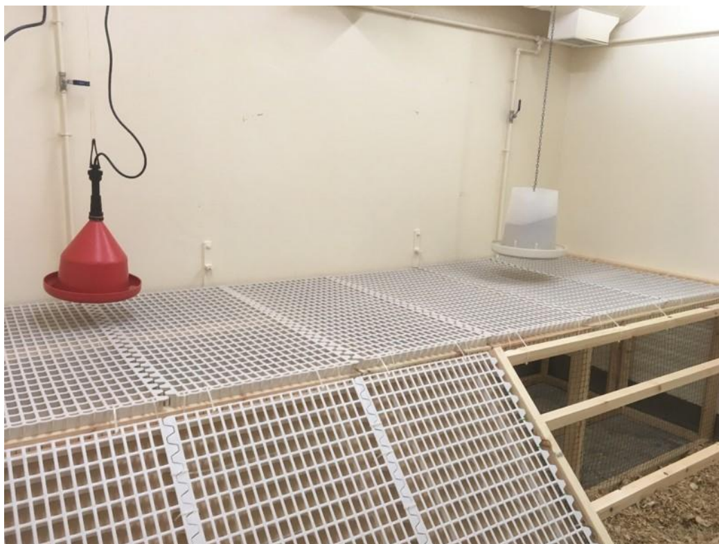
Figure 2-5. The raised area in the group testing room. Grid ramp (GR) on the left and ladder ramp (LR) on the right. Raised slatted area 90cm high with ramp angles of 45°.
