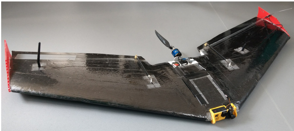
Figure 3.4: The RiteWing Zephyr II, used to scout the ability of drones to be used at Fuego. With the exception of a GoPro Hero 3 camera, no additional sensors were mounted.
