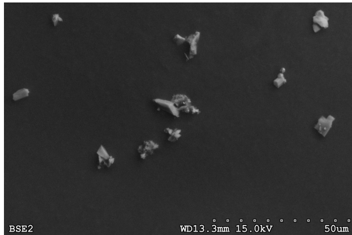
Figure 5.6: SEM stub imaging results, showing ash collected during Flight B8.
