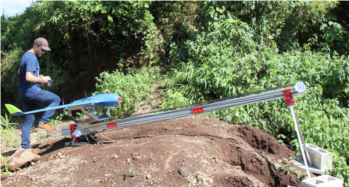
Figure 4.6: The catapult system used for launching the Skywalker X8, being operated on Trip B by the Author.
