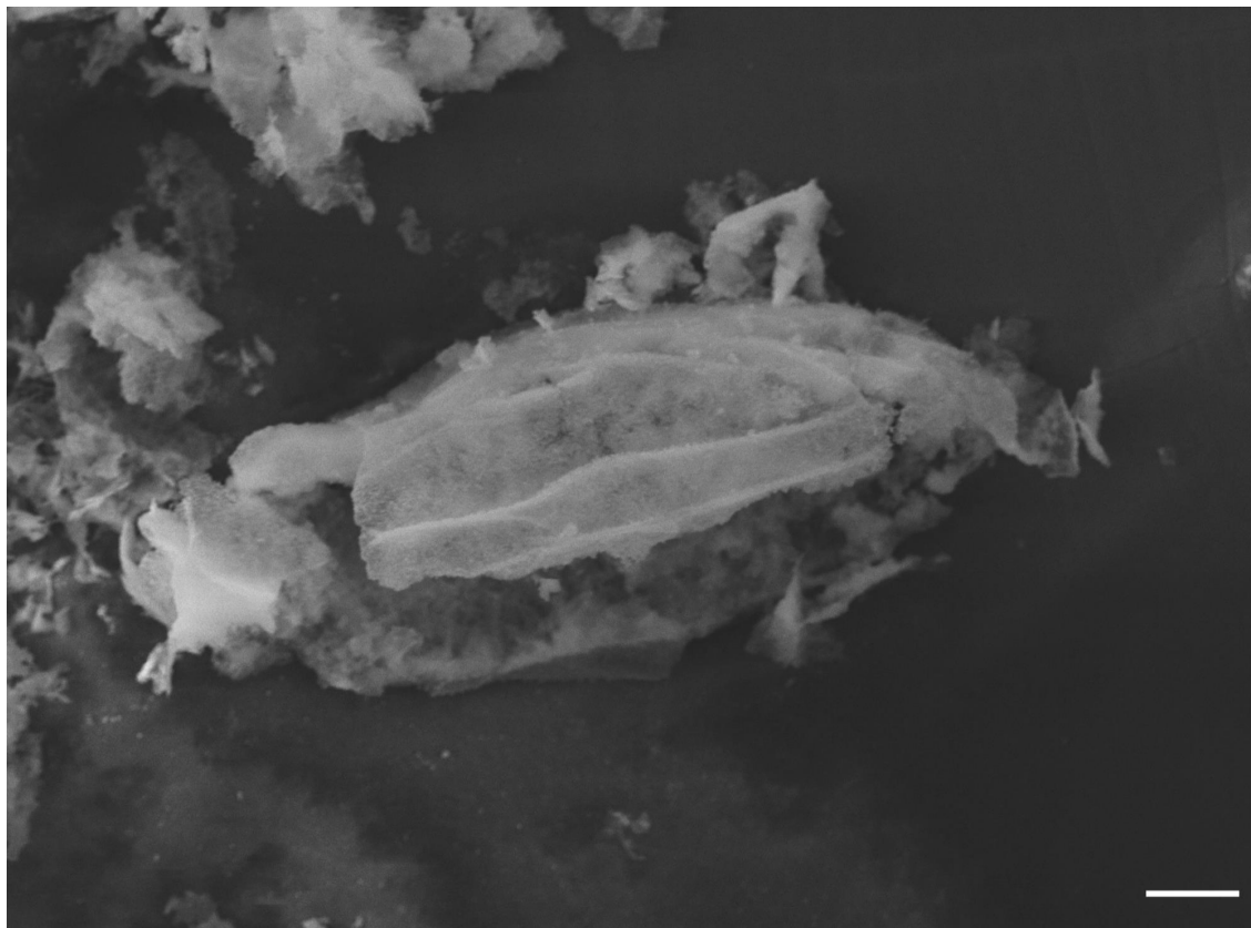
FIGURE A.6. Colloidosomes were formed via handshaking with aqueous phase pH 7. After crosslinking with TMOS and transfer to water, SEM samples were prepared by lyophilisation. Scale bar shows 10 \mu\text{m} .
