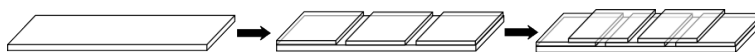
FIGURE 2.1. A scheme showing how channel slides are formed from glass slides and cover slips. Cover slips were stuck in place using UV cured glue.
