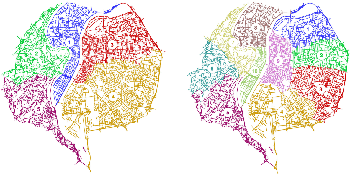
Figure 5.1 The Lyon road network partitioned into five and ten reservoirs respectively. Reproduced from [9], by Mariotte et al. (corresponding figure 4 in their paper).
