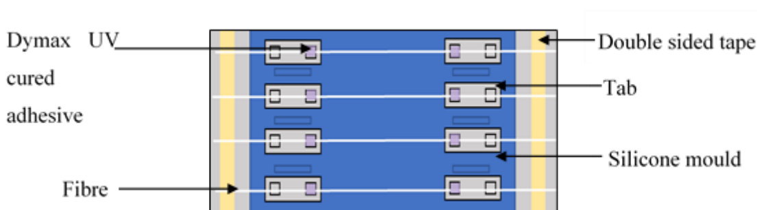
Figure 51: Schematic of the setup used to prepare the single fibre specimens.
