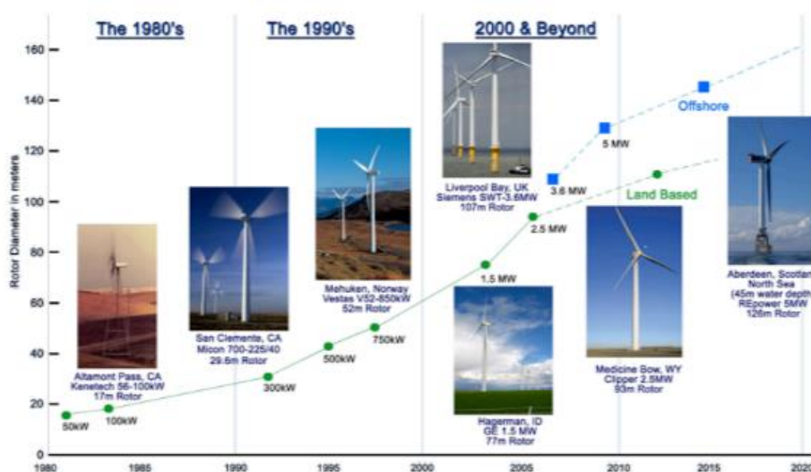
Figure 6: Development of wind turbine blades from 1980s to 2020 (predicted). Taken with permission from [45].
