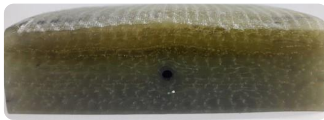
Figure 74: Photograph of sectioned cured GFRP laminate with central vasculature.
