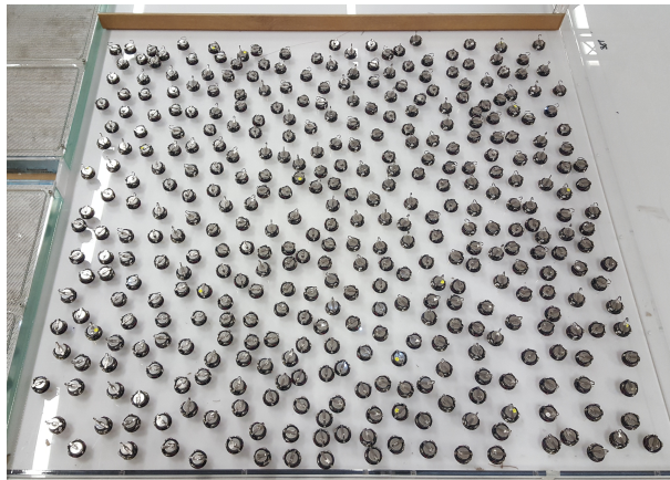
Figure 4.12: 1.2 m 2 Arena used for experiments in which Kilobots interact while moving amongst one another.
