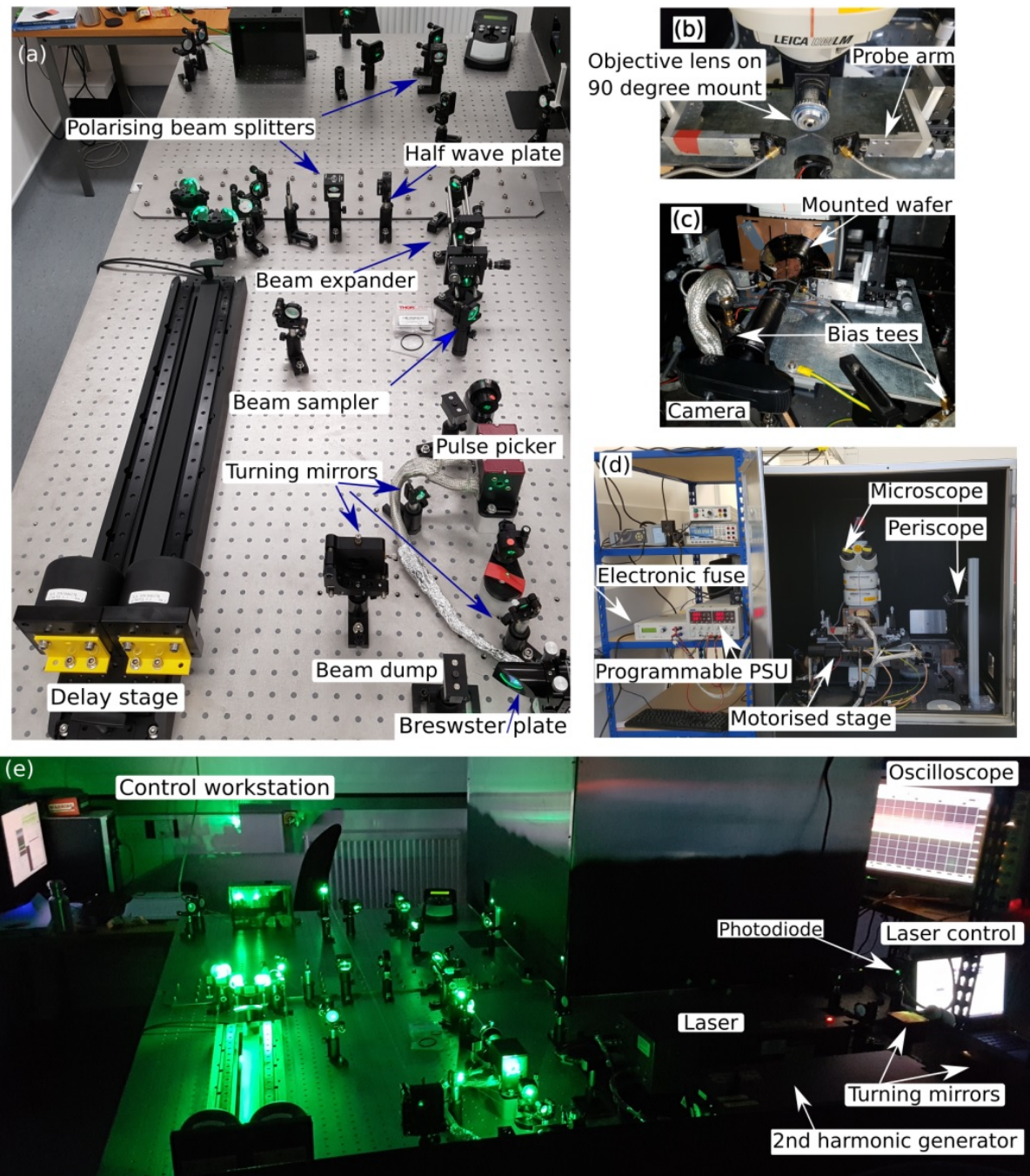
Figure 3.6: Pulsed femto-second laser setup constructed for this work. (a) In order of propagation: beam enters at bottom right through half wave plate and Brewster plate assembly for attenuation control. Pulse picker for pulse repetition frequency (PRF) control. Beam sampler diverts small fraction of beam towards photodiode for monitoring. A half wave plate controls the beam polarisation prior entering the first polarising beam splitter. Part of the beam continues into the delay line, and is then recombined with the undelayed part of the beam at the second polarising beam splitter. (b) microscope objective lens mounted on 90^\circ mirror cube. GSG probes mounted on three-axis mounts. Camera for wafer top side imaging is visible at the bottom of the image. (c) wafer in 90^\circ mount positioned for testing. Bias tees and semi-rigid coaxial connections to probes on custom made magnetic microscope stage plate. (d) Enclosure with adjacent instrumentation rack. (e) Setup in use.
