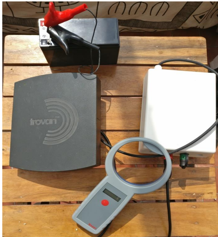
Figure 6.2. Trovan antennae and PIT-tag reader plus car battery power pack © J. Nightingale.
