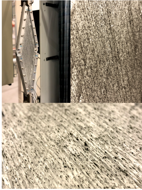
Figure 5.8: Clockwise from top left: Specimen sheared to \theta = 30^\circ prior to dismounting, close up of the speckle pattern, and a close up of the surface surface deformations accompanying shearing.
