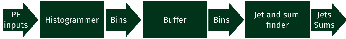
Figure 5.3: Diagram showing how the FPGA version of the jet and sum algorithm was organised.
