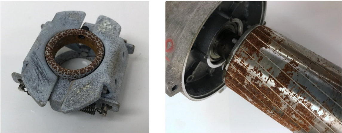
Figure 2.4: Examples of corrosion present within the centrifugal switch (l) and stator (r) of motor M2.
