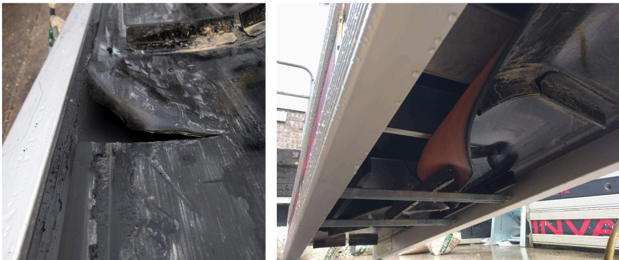
Figure 11.16: Deformation of System 2's belt as a result of lateral damage, folding under (l) and becoming trapped underneath the bed (r).
