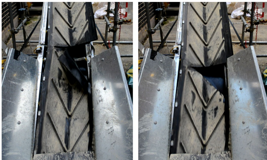
Figure 9.31: Examples of loose belt material folding backwards (l) and under itself (r) as a result of seeded lateral damage.
