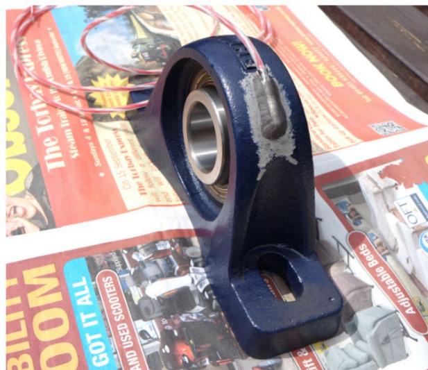
Figure 4.3: An example of an RTD bonded to a bearing.
