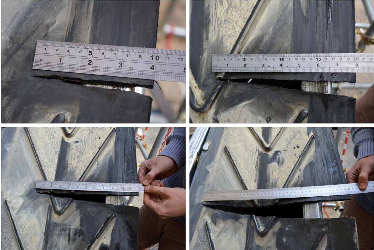
Figure 9.28: The progression of seeded belt damage. Clockwise from top left: 10cm, 20cm, 30cm, 40cm.
