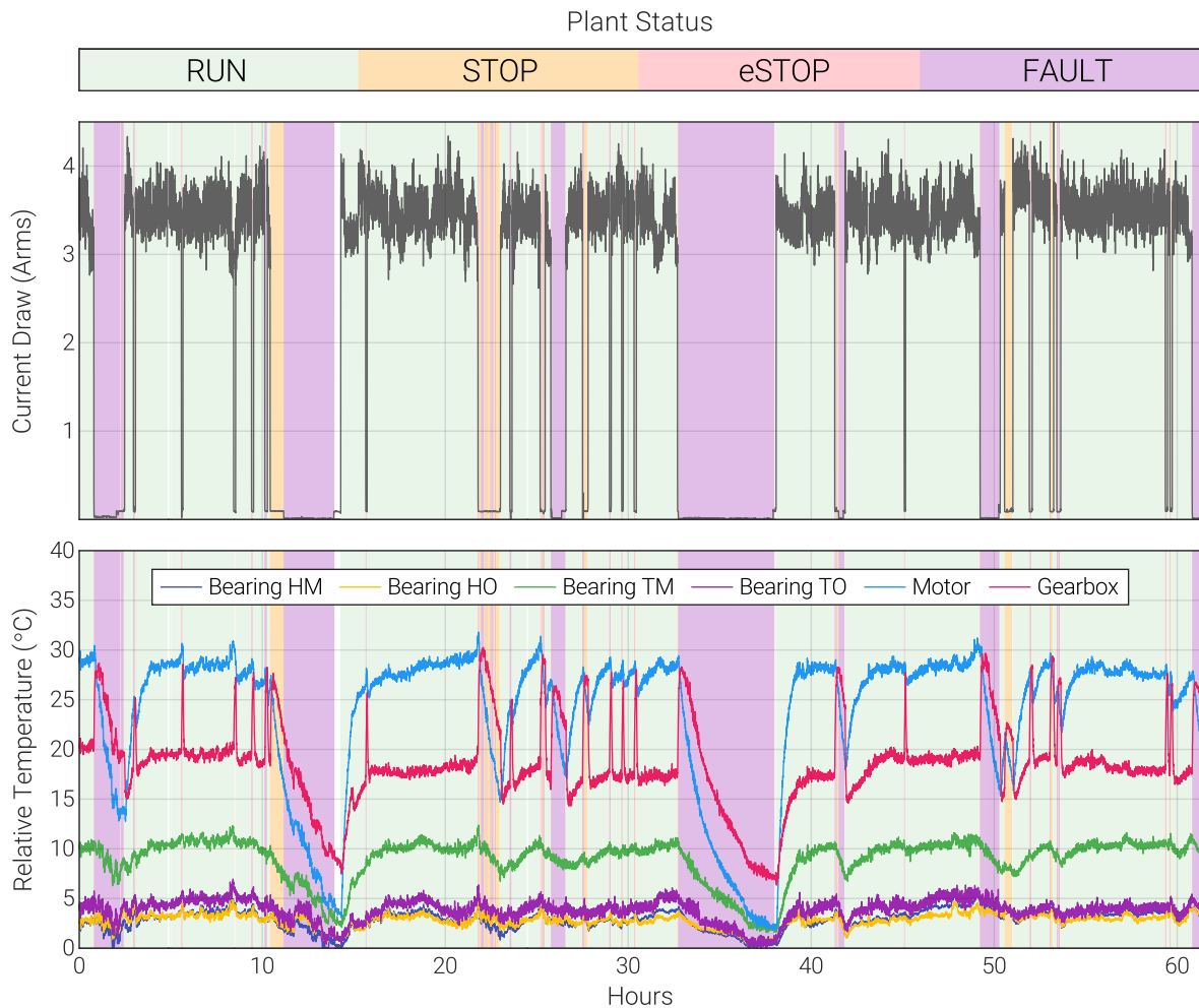
Figure 4.4: Illustrative example of component temperature and motor current draw data as acquired during the monitoring trial. Note, the overall Plant status is also shown.
