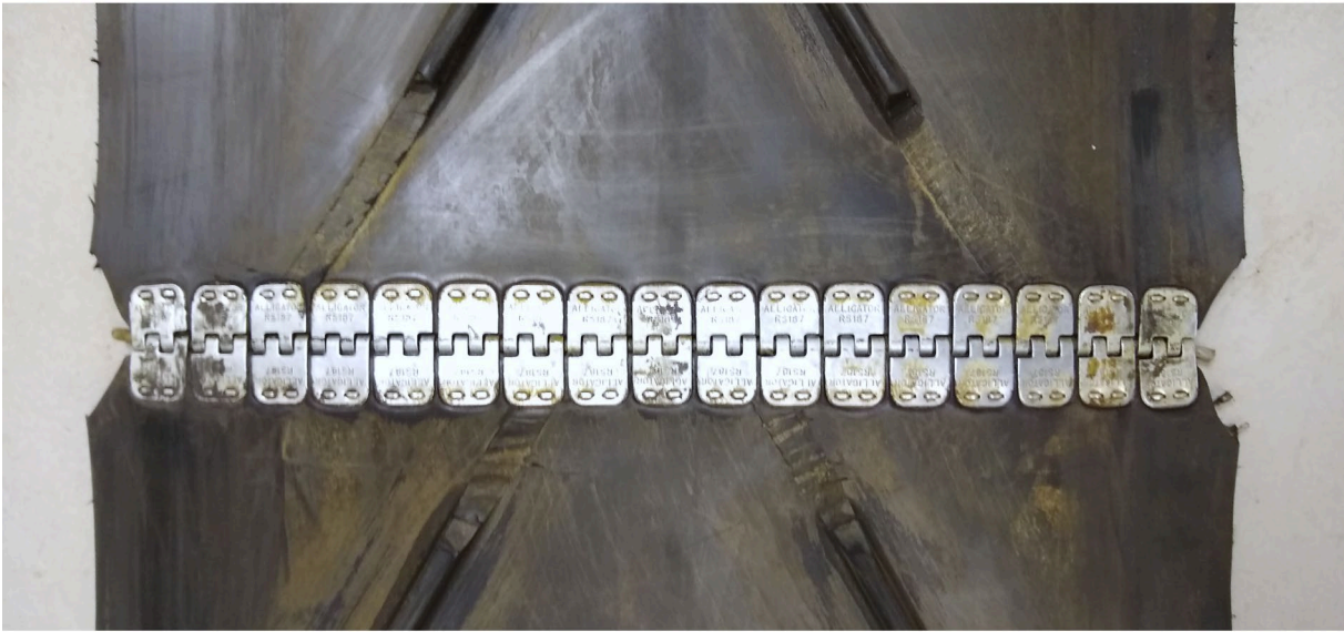
Figure 8.4: Hinged-style mechanical fastening of belt ends within the System. Note the removed sections of chevron material on either side of the splice.
