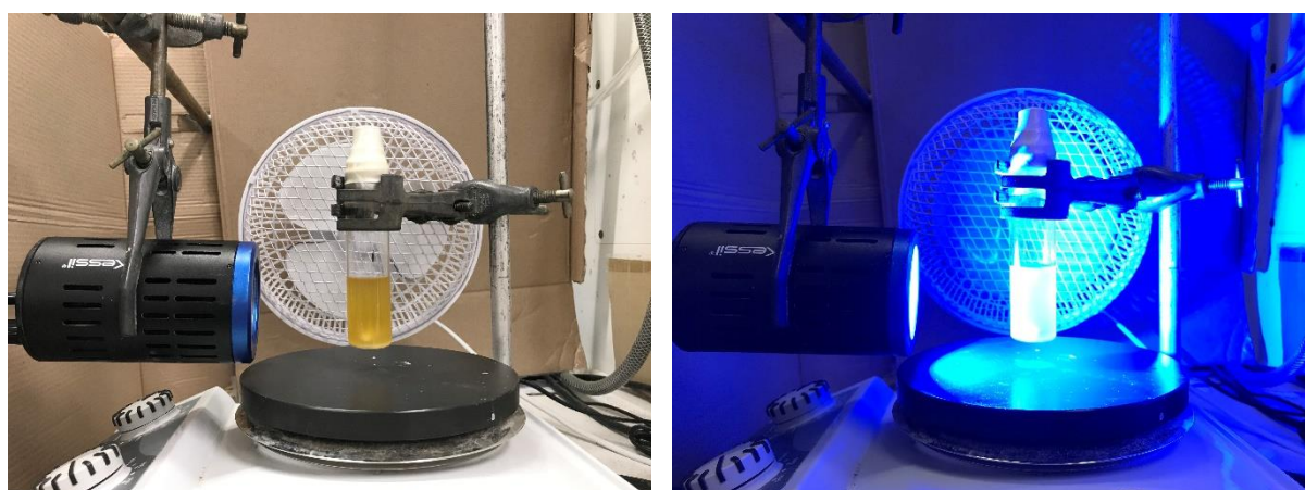
Figure S 5. Photoredox reaction set-up for the conjunctive cross-coupling of vinyl boronic esters.
