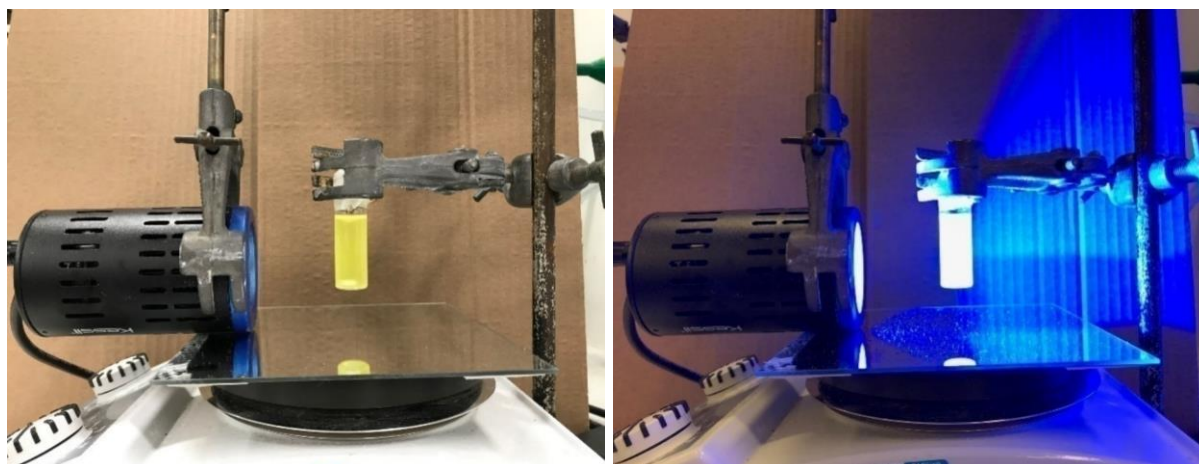
Figure S 3. Photoredox reaction set-up for the synthesis of cyclopropyl boronic esters.
