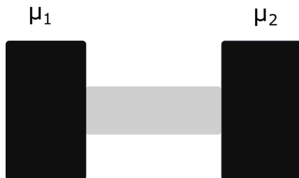
FIGURE 1.1. A 1D wire, connecting two reservoirs of potential \mu_1 and \mu_2 adiabatically, as described in Section 1.2 to determine the conductance in a mesoscopic system.
