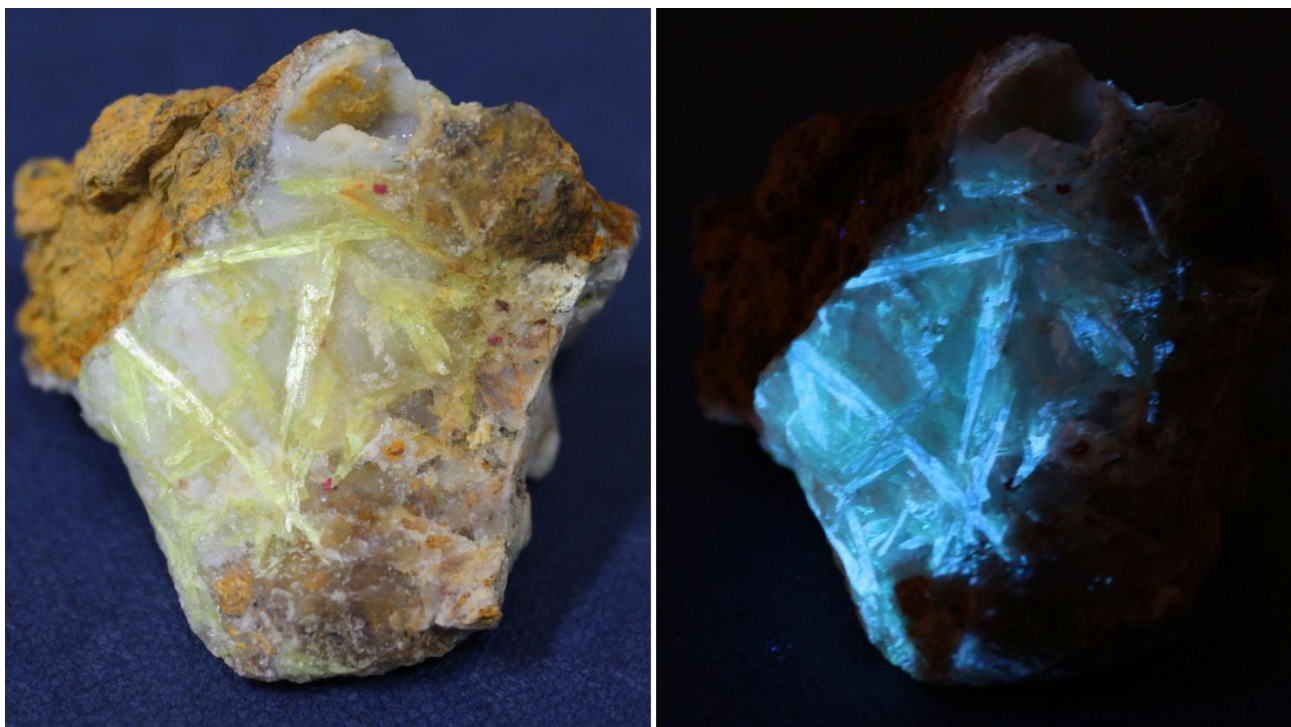
Figure 4.3: Left: Karpatite crystals (green) within a quartz vein (white). Right: The same crystals under UV illumination.
